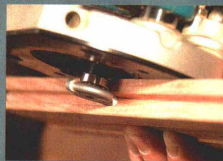
Router cuts new groove to mate floor and border. Using a top-bearing router bit, the author can cut a groove and mate two boards groove to groove with a spline.
