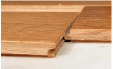
**Create a factory end.** With a slot-cutting bit in a router, restore the tongue or groove on the end of the board. To restore the factory bevel, make a few passes on the edge of the board with a palm sander.
